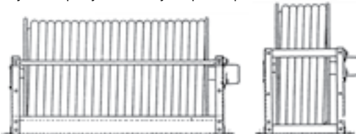
"FM" Floor-Ceiling Mount (Drag) All SP & DP Series are shipped in this position unless specified
