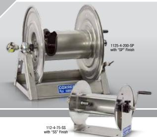
COXREELS® SS Series "Stainless Steel" hand crank hose reels have similar features to their related series, but are constructed of high quality electro-polished or unpolished as manufactured stainless steel with stainless steel fluid paths. They offer clean, non-corrosive performance in applications that require it, such as food and chemical processing, marinas, and anywhere that rust, corrosion and contamination thrive.
