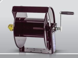
**COXREELS®** SM Series "Swivel Mount" hand crank hose reels swivel on demand in the direction your work takes you and locks in eight different positions as desired. Like the 100 Series, the SM Series is lightweight, compact and versatile with a working pressure up to 4,000 PSI. The "U" shaped base and hose control bar together add strength and rigidity while keeping the hose from slipping off the side discs. Add the SMK-202 wall mount bracket for swiveling mounted positions.
