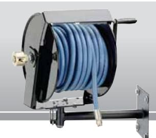
COXREELS® SM Series "Swivel Mount" hand crank hose reels swivel on demand in the direction your work takes you and locks in eight different positions as desired. Like the 100 Series, the SM Series is lightweight, compact and versatile with a working pressure up to 276 BAR. The "U" shaped base and hose control bar together add strength and rigidity while keeping the hose from slipping off the side discs. Add the SMK-202 wall mount bracket for swiveling mounted positions.
